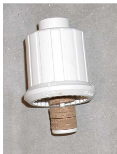
Figure 4. The expanding material of a shut-off device is visible in this photo of the cap removed from a device similar to the one in figure 3.
